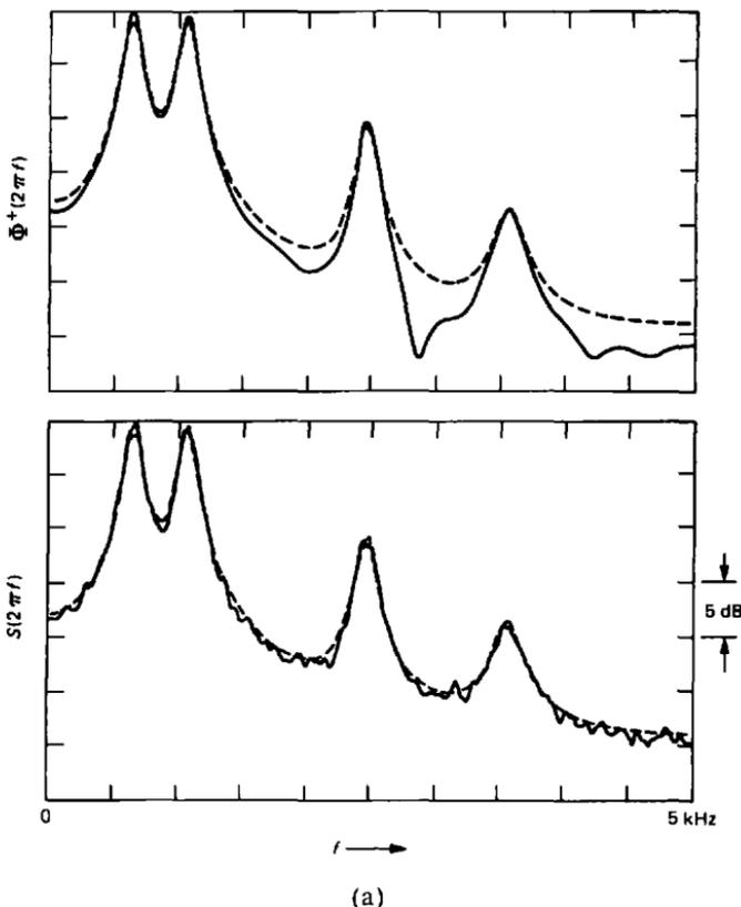
Fig. 7a—The specified spectral density is a typical spectral shape for the vowel /a/. On the top is  $\Phi(\omega)$  for the required  $\{x\}$  process. On the bottom is the plot estimated from a 25,000-sample sequence of the generated process. The dotted line in each case is the specified spectral density.
