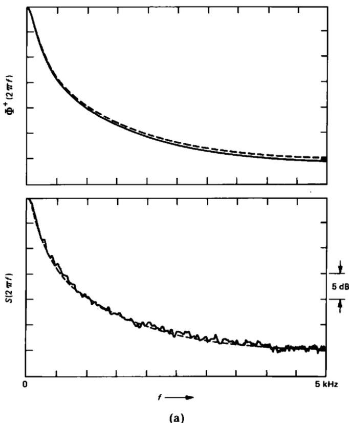
Fig. 6a—On the top the spectral density  $\Phi(\omega)$  required for the  $\{x\}$  process and on the bottom the spectral density estimated from a 25,000-sample sequence. The spectral density specified is the same as in Fig. 5.
