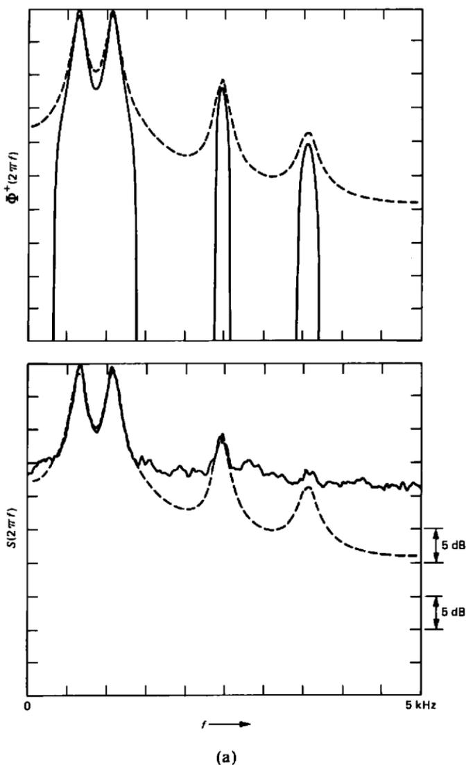
Fig. 9a—The specified spectral density is a typical spectral shape for the vowel /a/ for a process with a binary distribution. On the top is  $\Phi(\omega)$  for the required  $\{x\}$  process. On the bottom is the plot estimated from a 25,000-sample sequence of the generated process. Note that  $\Phi(\omega)$  had to be corrected to  $\Phi^+(\omega)$ , as shown in eq. (15).
