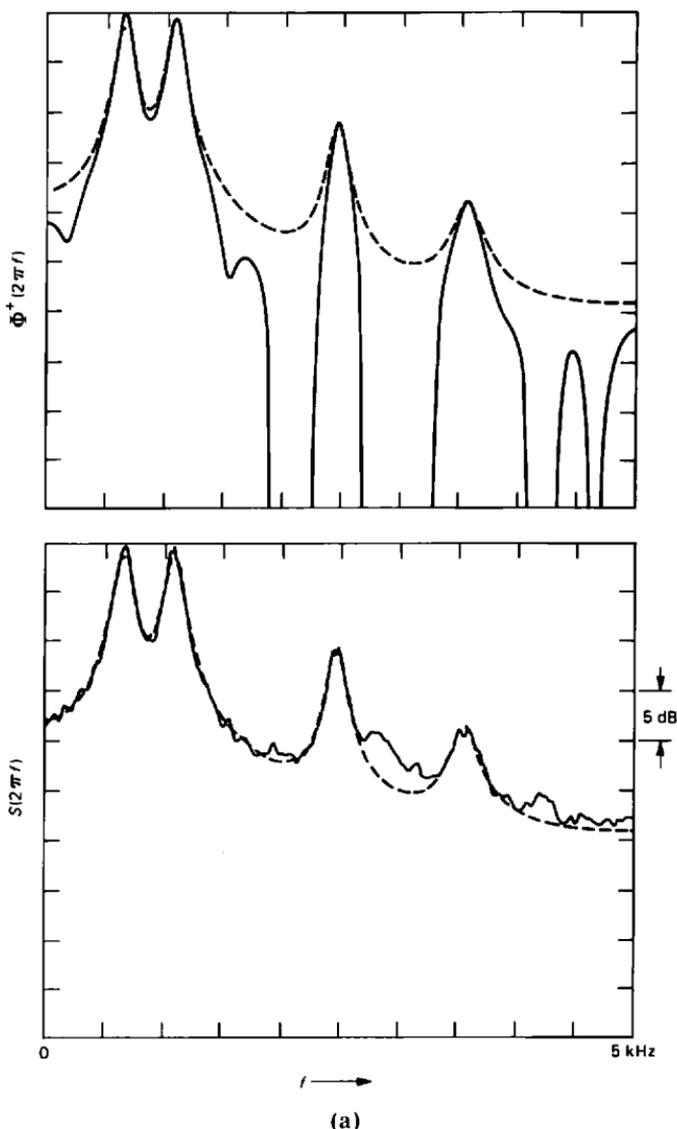
Fig. 8a—The specified spectral density is a typical spectral shape for the vowel /a/ for a process with a gamma probability distribution. On the top is  $\Phi(\omega)$  for the required  $\{x\}$  process. On the bottom is the plot estimated from a 25,000-sample sequence of the generated process. Note that  $\Phi(\omega)$  had to be corrected to  $\Phi^+(\omega)$ , as shown in eq. (15).
