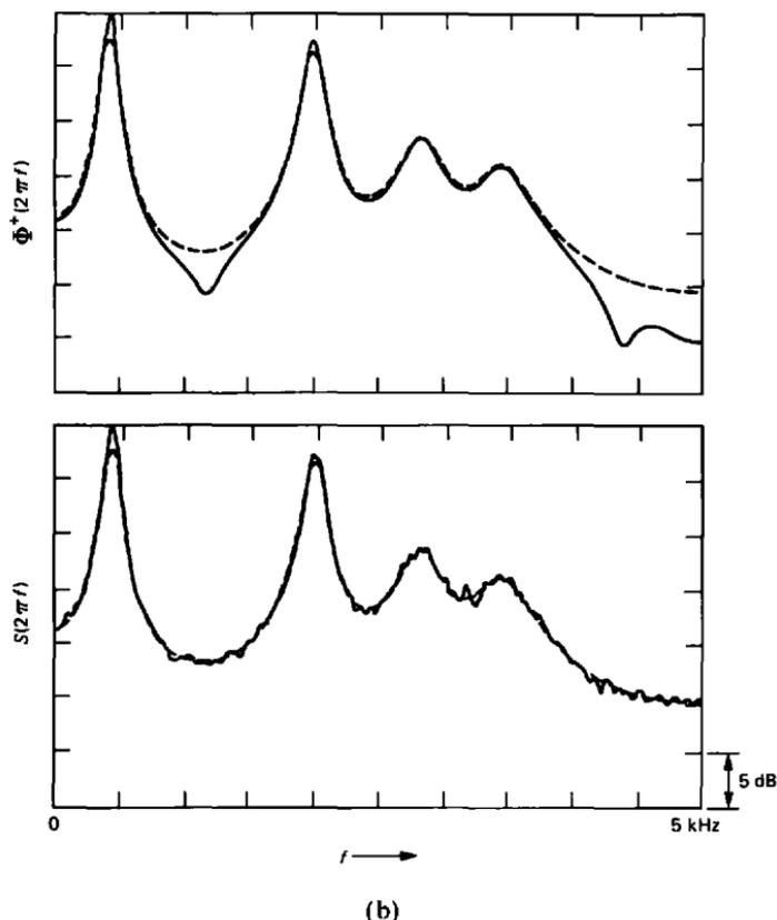
Fig. 7b—Same as Fig. 7a but for the vowel /e/. The plots are for a process with a uniform probability density.
