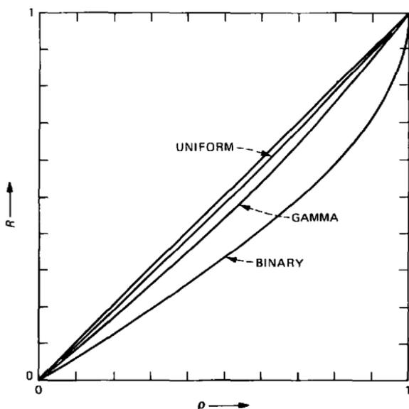
Fig. 4—The relationship between the autocovariance ( $R$ ) at the output and ( $\rho$ ) at the input of the nonlinearity appropriate to the generation of the three desired probability distributions. The unmarked line is  $R = \rho$ . Since the functions have odd symmetry, only the range of positive covariance values is shown.
