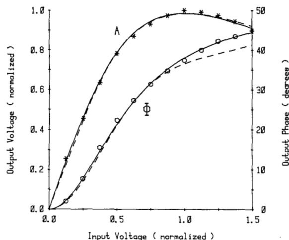
Fig. 2. TWT amplitude (\*) and phase (o) data of Berman and Mahle [5]. The solid lines are plotted from (3) and (4), and the dashed lines from the Berman-Mahle [5] phase formula, and from the Thomas-Weidner-Durrani [7] amplitude formula.
