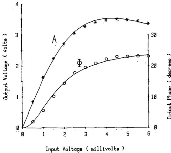
Fig. 4. TWT amplitude (\*) and phase (o) data obtained from Hetrakul and Taylor [11]-[13] through the use of (6). The solid lines are plotted from (3) and (4).
