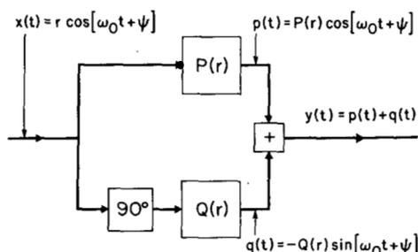
Fig. 1. Quadrature nonlinear model of a power amplifier.
