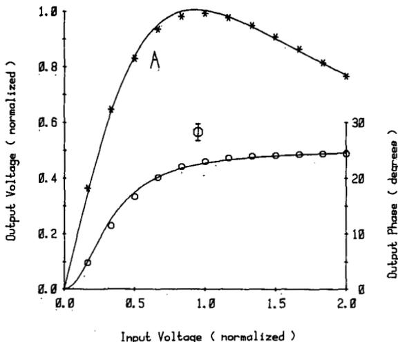
Fig. 6. TWT amplitude (\*) and phase (o) data of Kaye, George, and Eric [9]. The solid lines are plotted from (3) and (4).
