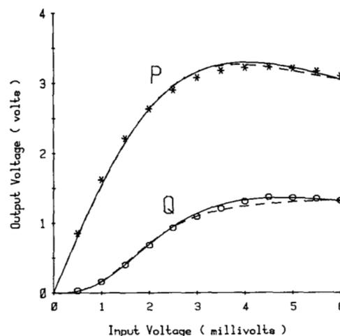
Fig. 3. TWT in-phase (\*) and quadrature (o) data of Hetrakul and Taylor [11]–[13]. The solid lines are plotted from (7) and (8), and the dashed lines from their own formulas [11]–[13].
