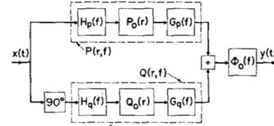
Fig. 7. Proposed frequency-dependent quadrature model of a TWT amplifier.  $P_0(r)$  and  $Q_0(r)$  are frequency-independent envelope nonlinearities given in (29) and (30); the  $H$ 's and the  $G$ 's are real linear filters whose frequency responses are defined in (25)–(28), and  $\Phi_0(f)$  is a linear all-pass network whose phase response is defined in (22).
