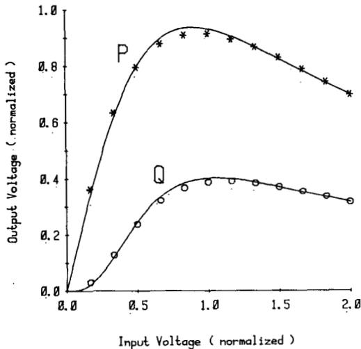
Fig. 5. TWT in-phase (\*) and quadrature (o) data of Kaye, George, and Eric [9]. The solid lines are plotted from (7) and (8).
