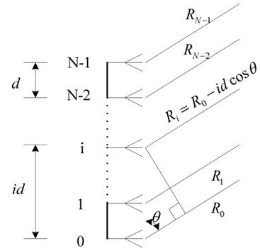
Fig. 2. An antenna array with  $N$  antenna elements.
