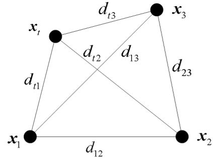
Fig. 7. A fully-connected planar quadrilateral in sensor networks.
