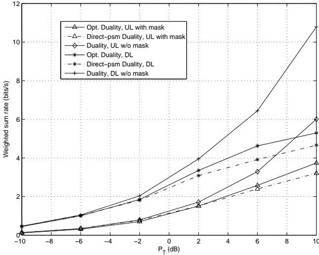
Fig. 3. Weighted sum rate vs. total transmit power  $P_T$  for the duality schemes in CRN uplink and downlink transmissions.  $N_c = 16$ ,  $K = 6$ , and  $P_{\text{COP}} = 0.5$ .
