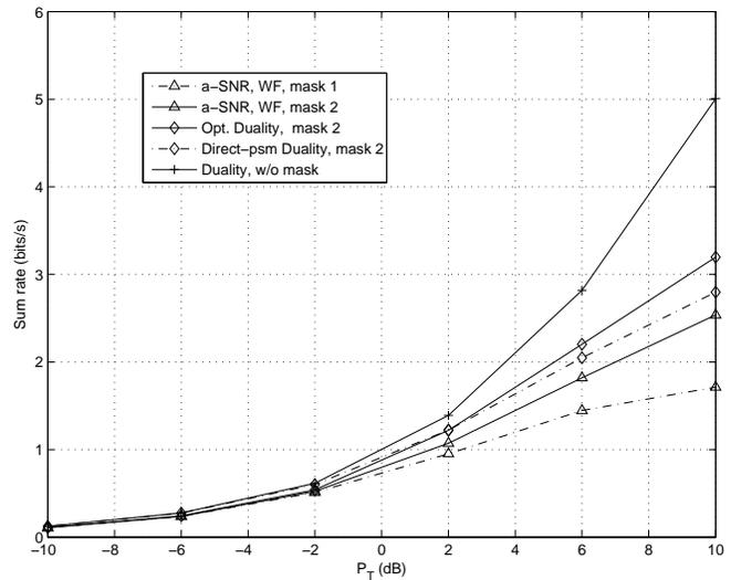
Fig. 2. Sum rate vs. total transmit power  $P_T$  for the duality and the  $a$ -SNR schemes in CRN uplink transmission.  $N_c = 16$ ,  $K = 6$ , and  $P_{\text{COP}} = 0.5$ .
