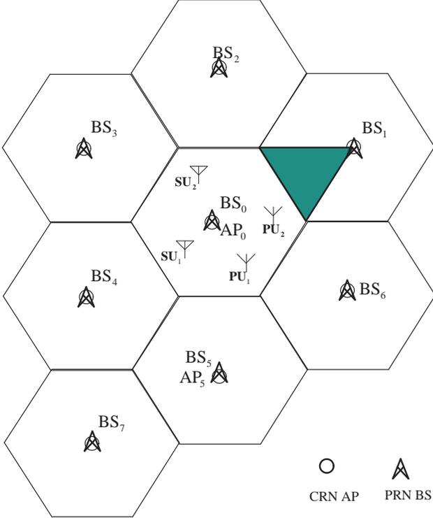
Fig. 1. System model of multicell PRNs and multicell cellular CRNs.
