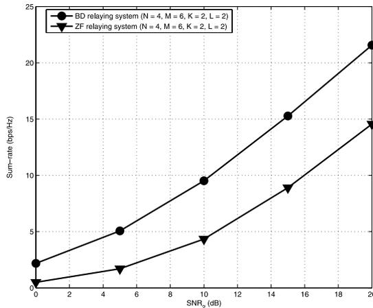
Fig. 3 Sum-rate v.s.  $SNR_2$  at relay node  $M = 6$ .
