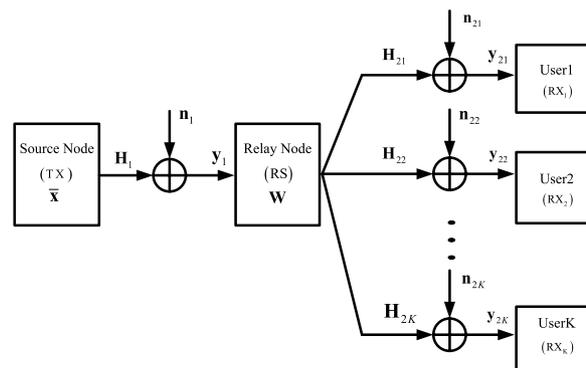
Fig. 1 Model of MU-MIMO relay system.
