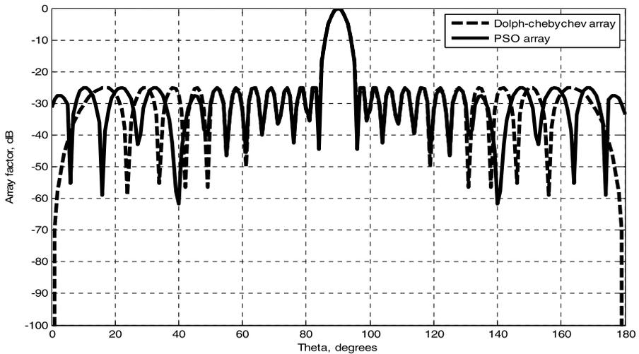
**Fig. 4** The resulting PSO and Dolph–Chebyshev array factors (24 elements)
