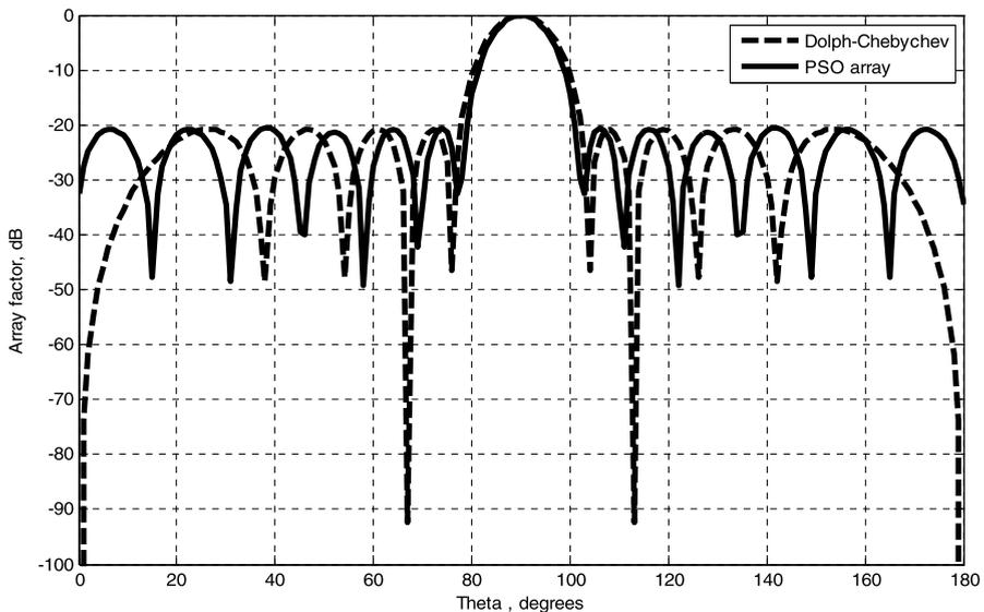
**Fig. 7** The position perturbation resulting array factor for the broadside case (10 elements)
