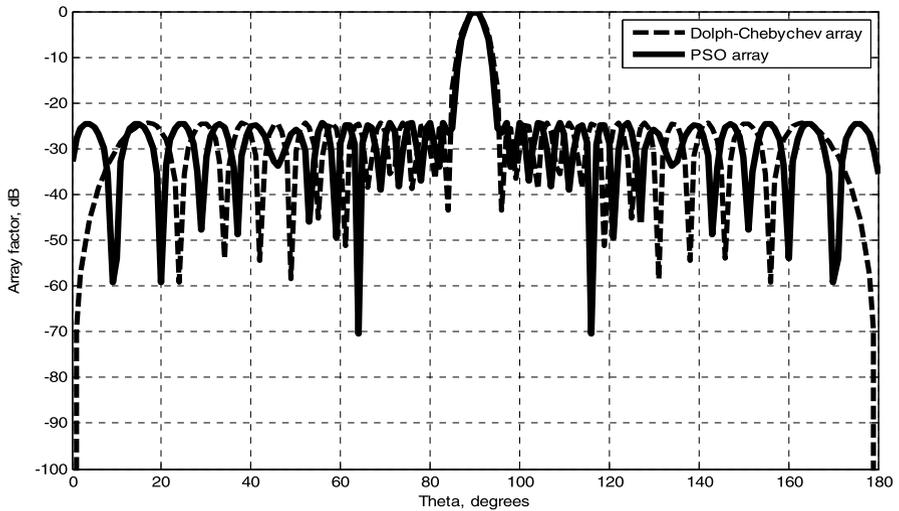
**Fig. 9** The position perturbation resulting array factor for the broadside case (24 elements)
