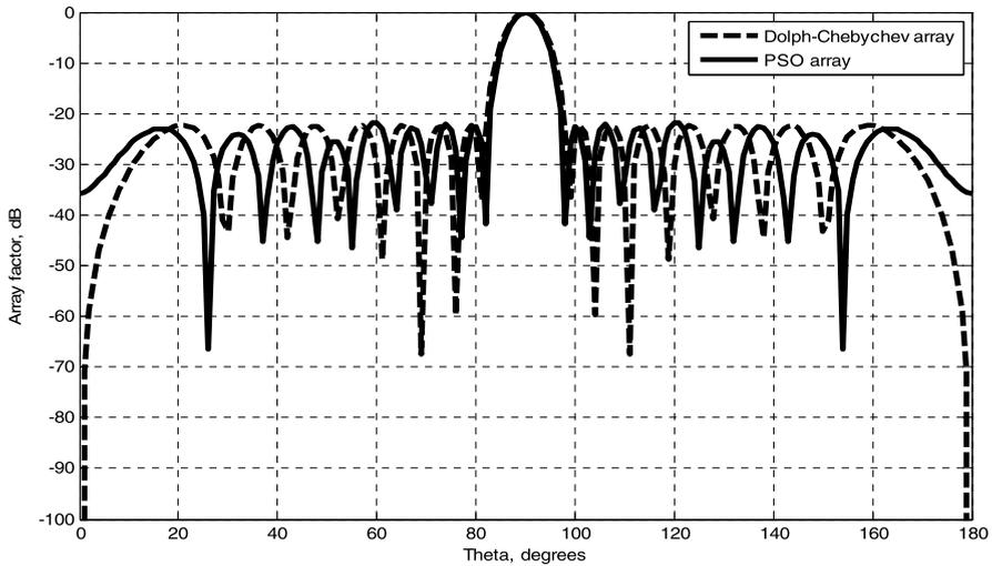
**Fig. 8** The position perturbation resulting array factor for the broadside case (16 elements)
