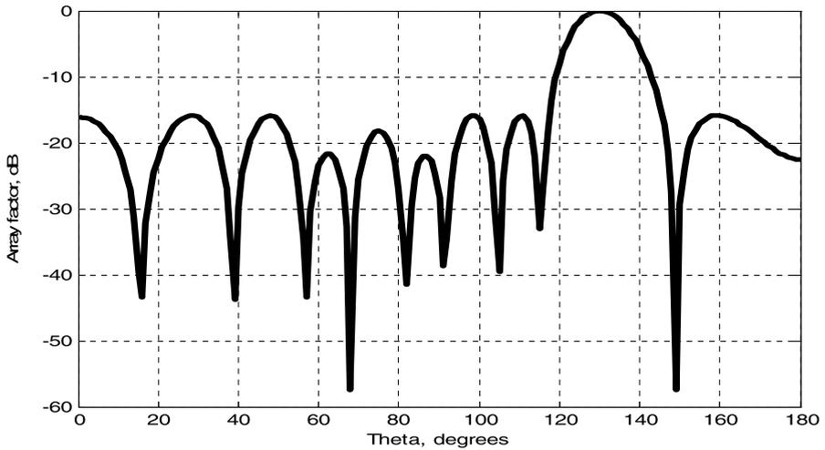
**Fig. 11** The perturbation array factor with the main beam steered towards  $130^\circ$  (10 elements)
