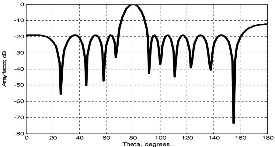
**Fig. 10** The perturbation array factor with the main beam steered towards  $80^\circ$  (10 elements)
