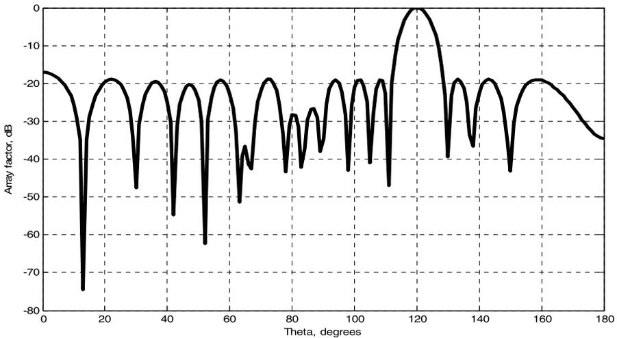
**Fig. 6** The resulting array factor with the main beam steered towards  $120^\circ$  (16 elements)
