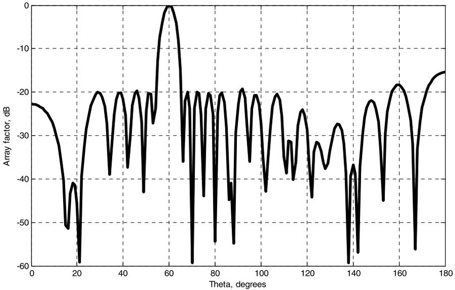
**Fig. 5** The resulting array factor with the main beam steered towards  $60^\circ$  (24 elements)
