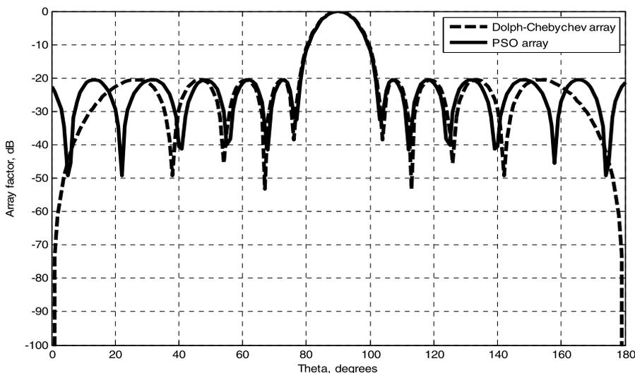
**Fig. 2** The resulting PSO array pattern along with the Dolph–Chebychev array (10 elements)
