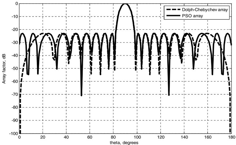
**Fig. 3** The resulting array factor and the Dolph–Chebychev one for comparison (16 elements)
