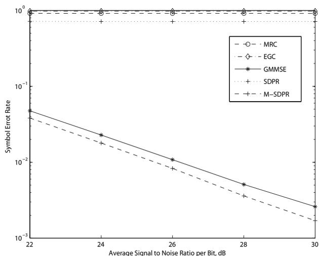
Fig. 3. SERs of the 64-QAM system (example three).
