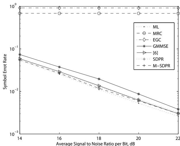
Fig. 1. SERs of the 16-QAM system (example one).
