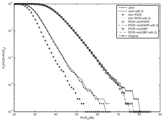
**Fig. 3** PICR performance of phase rotation based algorithms for OFDM systems with 16QAM.
