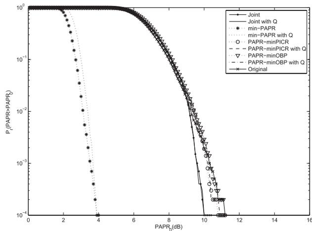
**Fig. 5** PAPR performance of phase rotation based algorithms for OFDM systems with 16QAM.
