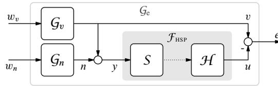
Fig. 11. Setup for SR with noisy measurements (Section X)
