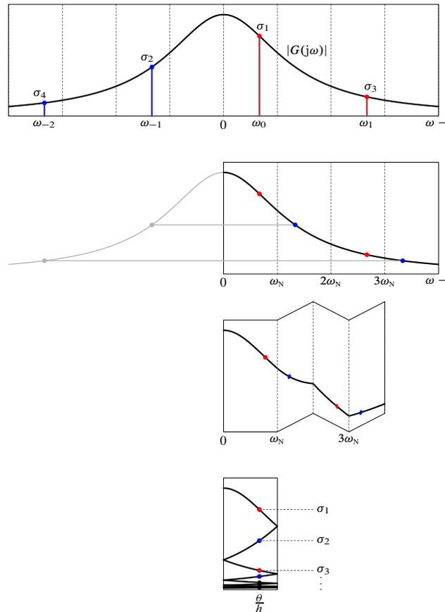
Fig. 4. Frequency folding for LCTI systems: at each  $\theta/h \in [0, \omega_N]$  the  $\check{G}(e^{j\theta})$  has countably many singular values  $\sigma_k = |\check{G}(e^{j\omega_k})|$ , modulo ordering
