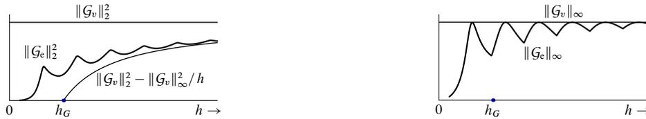
Fig. 7. Optimal  $\|\mathcal{G}_e\|_2^2$  (left) and  $\|\mathcal{G}_e\|_\infty$  (right) as a function of  $h$
