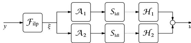
Fig. 9. Alternative implementation of a two-channel HSP
