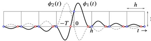
Fig. 10. Optimal hold functions for  $M = 2$  (Example 8.2)
