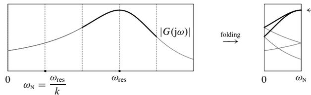
Fig. 6. Sampling at  $\omega_N = \omega_{\text{res}}/k$
