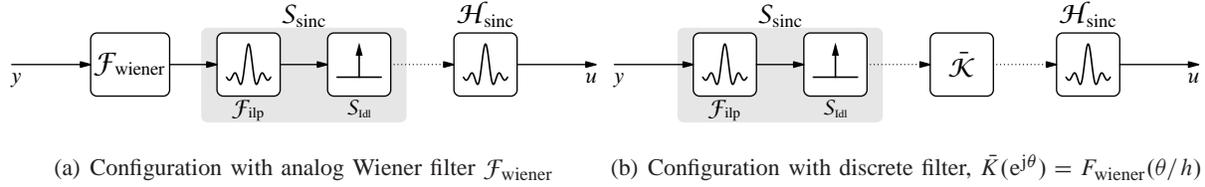
Fig. 12. The optimal HSP for SR with noisy measurements
