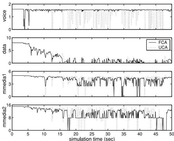
**Fig. 8** Simulation trace of the achieved utilities of voice, data and multimedia users in a typical simulation scenario.
