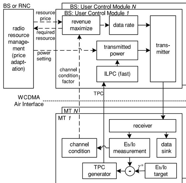
Fig. 4 Implementation structure of proposed utility-based radio resource allocation scheme and algorithms.
