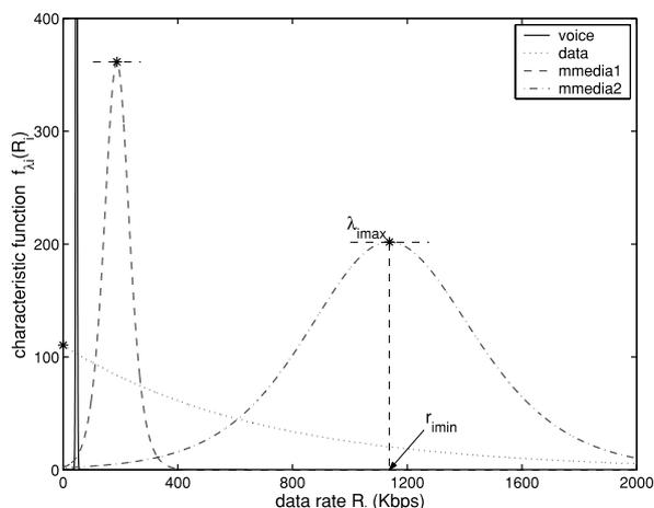
**Fig. 2** Characteristic functions of typical voice, data and multimedia traffic in system with  $\gamma^* = 1.55$  and  $E_s^* = 0.3425$ .
