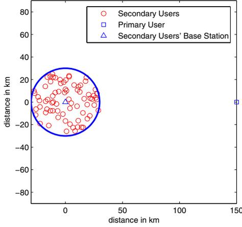
Fig. 1. Topology of Cognitive Radio Network.
