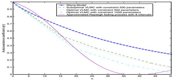
Fig. 4. Comparison of the auto-covariance coefficient among different VLMC channel models and the discretized fading process with 8 intervals in a Rayleigh fading process with normalized Doppler frequency 0.01
