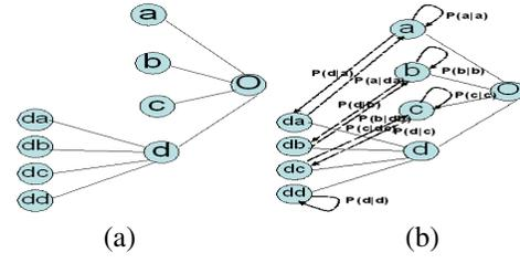
Fig. 1. (a) The context tree structure of the variable length Markov chain (b) The corresponding finite state machine of the context tree of (a).
