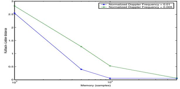
Fig. 2. The K-L distance between the Rayleigh fading channel and the estimate using the proposed fading partition scheme as a function of the number of fading samples.
