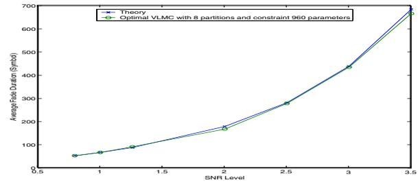
Fig. 5. Comparison of the average fade duration of Rayleigh fading obtained from theory and optimal VLMC when normalized Doppler frequency is equal to 0.01
