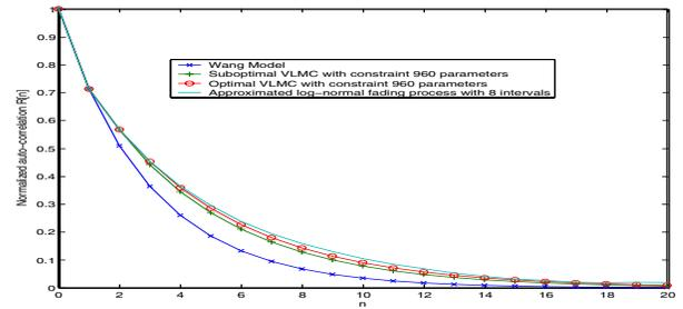
Fig. 3. The comparison of the normalized auto-correlation among different VLMC channel models and the discretized fading process under the log-normal fading process in sub-urban environments with  $\rho = 0.82$  and  $\sigma = 7.5$  dB with 8 intervals
