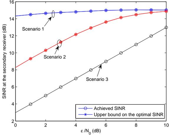
Fig. 3. SINR at the secondary receiver vs.  $\epsilon_k/N_0$  when  $K = 4$ .
