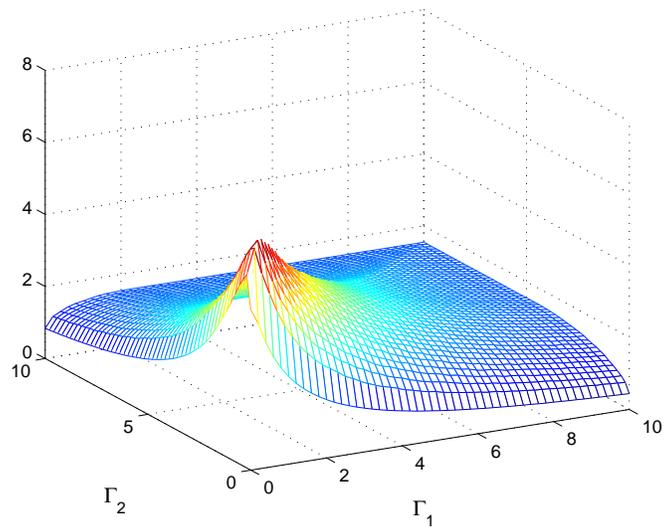
Fig. 3. The value of the function  $\min_{i=1,2} F_i(\Gamma_1, \Gamma_2)$  for  $M = N = 4$ ,  $K = 2$  single-antenna eavesdroppers, and  $P = 5$  dB.
