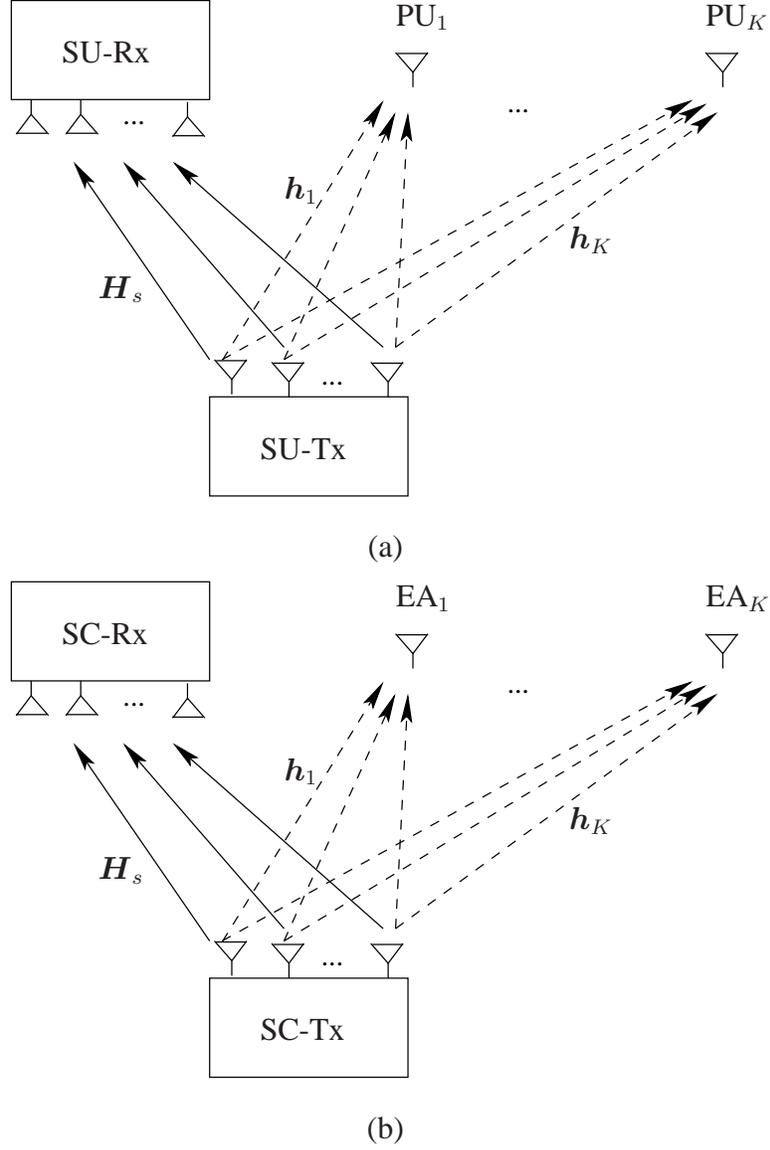
Fig. 1. The comparison of two system models: (a) the CR MIMO channel with  $K$  single-antenna PUs; and (b) the secrecy MIMO channel with  $K$  single-antenna eavesdroppers.
