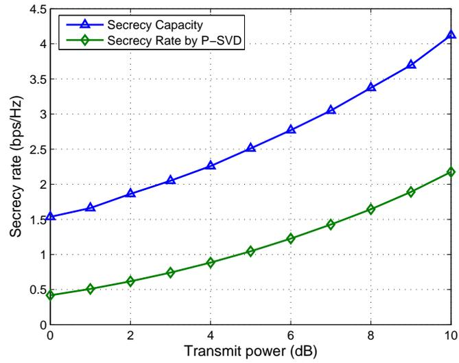
Fig. 4. Comparison of the secrecy capacity by Algorithm 2 and the secrecy rate by the P-SVD algorithm in [12] for  $M = N = 4$  and  $K = 1$  single-antenna eavesdropper.
