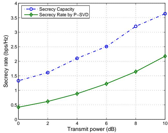
Fig. 2. Comparison of the secrecy capacity by Algorithm 1 and the secrecy rate by the P-SVD algorithm in [12] for  $M = N = 4$  and  $K = 2$  single-antenna eavesdroppers.
