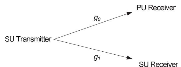
Fig. 1 Spectrum-sharing system model.
