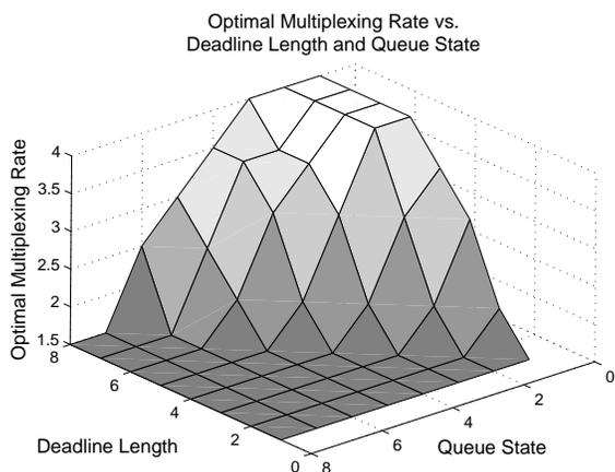
Fig. 8. Optimal multiplexing gain vs. queue state vs. deadline length  $k$  (SNR=10 dB).
