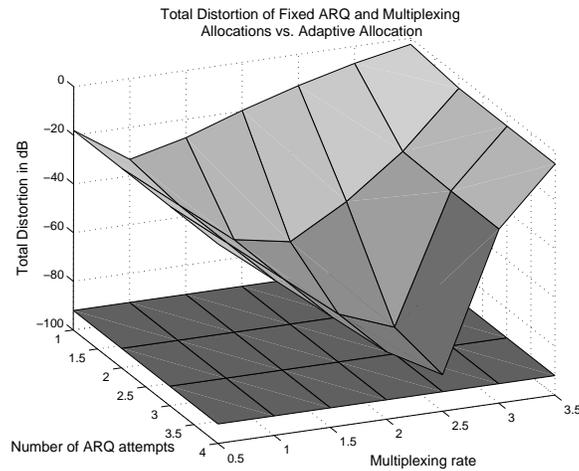
Fig. 9. Distortion for the fixed allocation problem vs. multiplexing gain vs. ARQ window size (SNR=10 dB).
