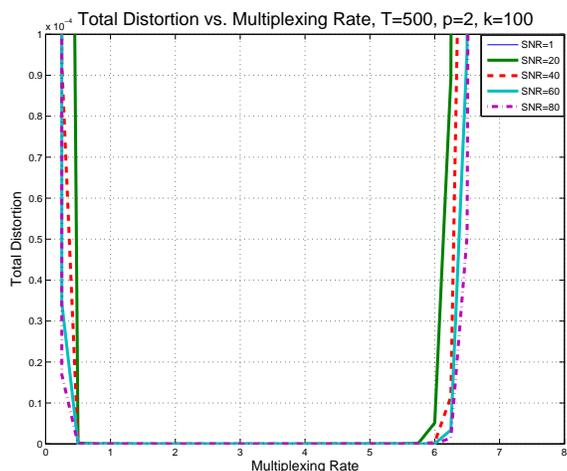
Fig. 5. Total distortion vs. number of antennas assigned to multiplexing in an  $8 \times 8$  system ( $T \gg k$ ).
