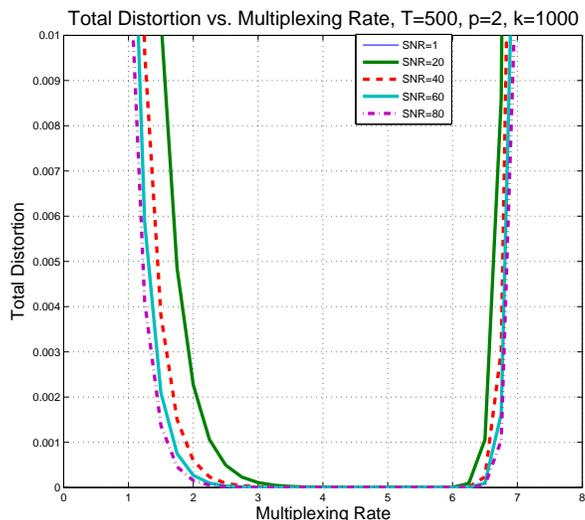
Fig. 4. Total distortion vs. number of antennas assigned to multiplexing in an  $8 \times 8$  system ( $T \approx k$ ).
