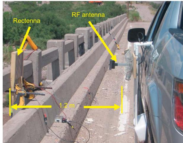
Fig. 15. Wireless energy transmission system field tested using ground vehicle as a mobile-host.
