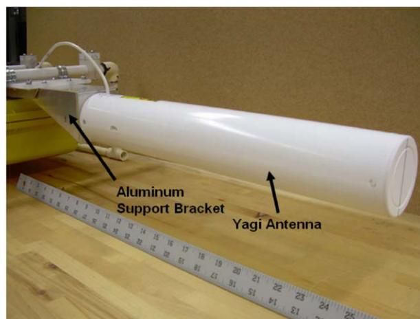
Fig. 5. Yagi antenna used to transmit RF energy.
