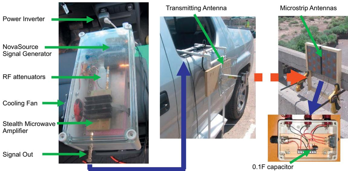
Fig. 9. An energy transmission system based on a ground vehicle.
