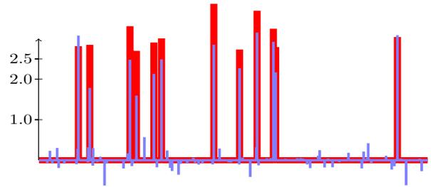
Fig. 1. Original Signal and Reconstruction from 100 measurements
