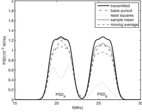
Fig. 2. True PSD transmitted by  $T_A$  and  $T_B$  and estimates obtained by four methods under consideration.
