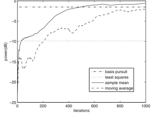
Fig. 3. Power of the estimates obtained with the four methods under consideration normalized to the power of the actually transmitted signals.
