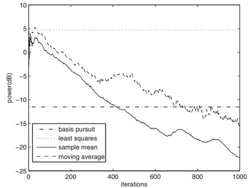
Fig. 5. Aggregate power of spatially spurious estimates normalized to the power of the transmitted signals.
