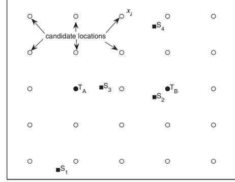
Fig. 1. Virtual network grid with 25 candidate locations and 2 actual transmitters.
