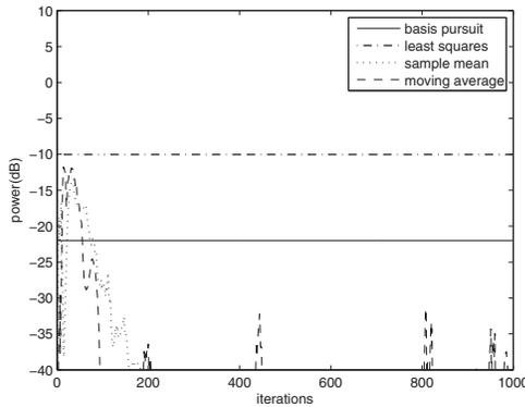
Fig. 4. Aggregate power of spurious estimates outside the transmission bands normalized to the power of the transmitted signals.
