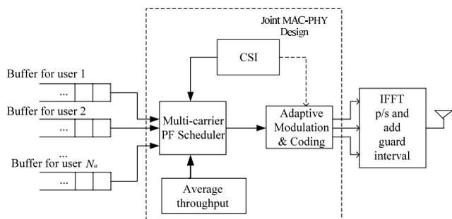
Fig. 1 Cross-layer scheduling model for OFDM systems.
