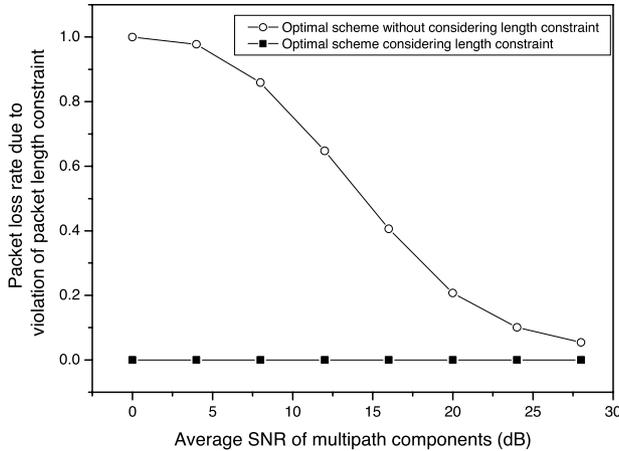
**Fig. 2** Packet loss rate due to violation of length constraint versus average SNR.
