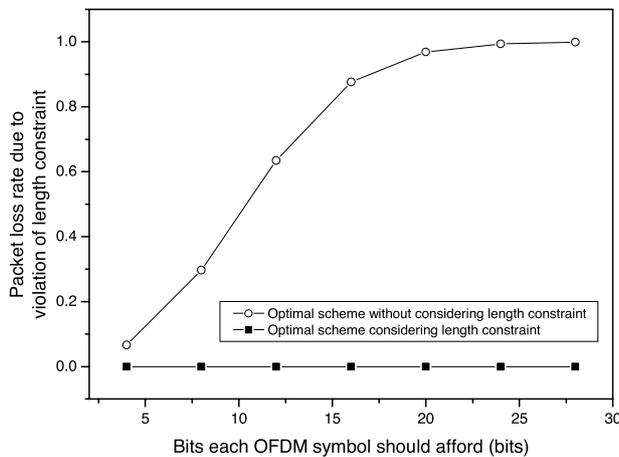
**Fig. 3** Packet loss rate due to violation of length constraint as a function of the number of bits each OFDM symbol should afford.
