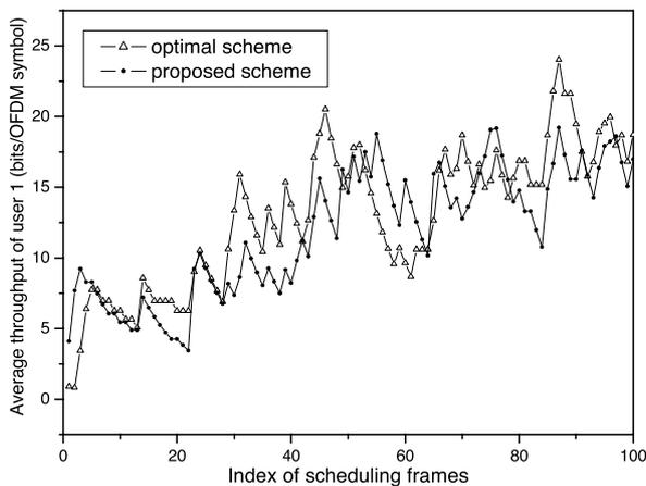
Fig. 5 User 1's average throughput with simulation time for the case of  $\overline{SNR}_1 = \overline{SNR}_2 = 10$  dB.
