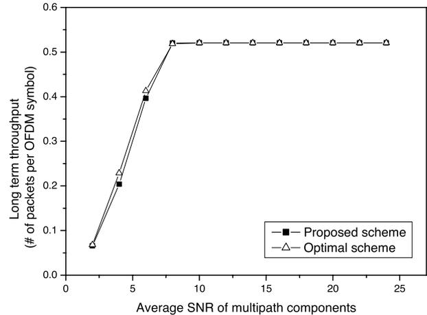
Fig. 6 User 1's long-term throughput versus average SNR.
