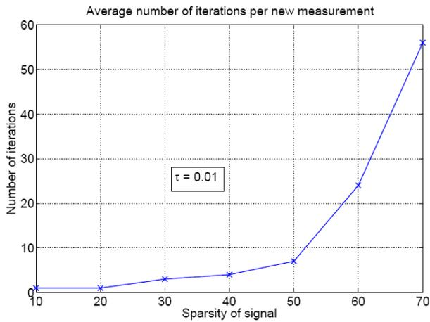
Fig. 4 Average number of homotopy steps with one new measurement at different sparsity levels. ( $n=256$ ,  $m=150$ )
