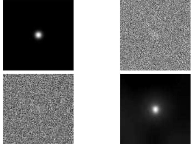
Fig. 9 **Top - left** : Input image of size  $128 \times 128$ . **Top - right** : First noisy input data  $x1$ . White Gaussian noise is added with SNR = .26dB. **Bottom-left** : Estimate from the average of 10 images compressed by JPEG with a compression rate  $\rho = 0.25$ . **Bottom-right** : Estimate from 10 pictures compressed by CS with a compression rate  $\rho = 0.25$ .
