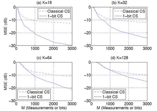
Fig. 2 Reconstruction quality from 1-bit measurements. [23]
