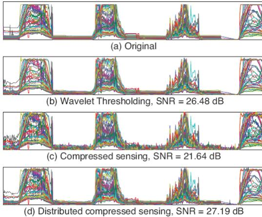
Fig. 7 Reconstruction of light intensity signals from 48 sensors with length  $N = 1024$ . (a) Original signals; (b) wavelet thresholding using 100 coefficients per sensor, average SNR = 26.48dB; (c) separate reconstruction of each signal using CS from  $M = 400$  random projections per sensor, average SNR = 21.64dB; (c) joint reconstruction of the signal ensemble using DCS from  $M = 400$  random projections per sensor, average SNR = 27.19dB.
