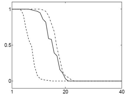
(a) Success rate vs. sparsity  $M = 1, \dots, 40$  for  $D = 100$ ,  $N = 40$ ,  $|c_k| = 1$  for  $k \in T$ , FFT.
