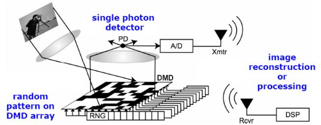
Fig. 5 Architecture of 1-pixel camera [34]
