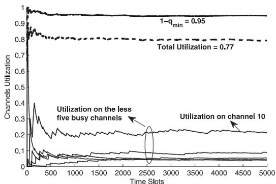
**Fig. 2** Channels utilization over time and maximum achievable utilization.
