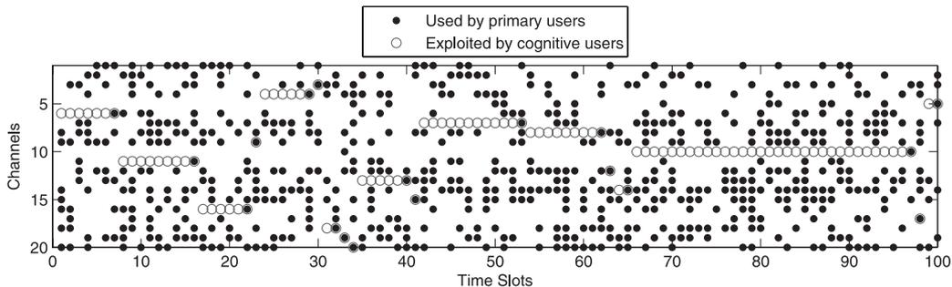
**Fig. 1** The exploited time slots by the cognitive user in 100 consecutive time slots using least failure rule.
