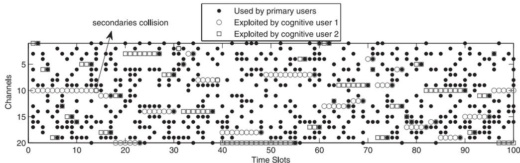
Fig. 3 The exploited time slots by  $M = 2$  cognitive users in 100 consecutive time slots using Alg. 1 independently.
