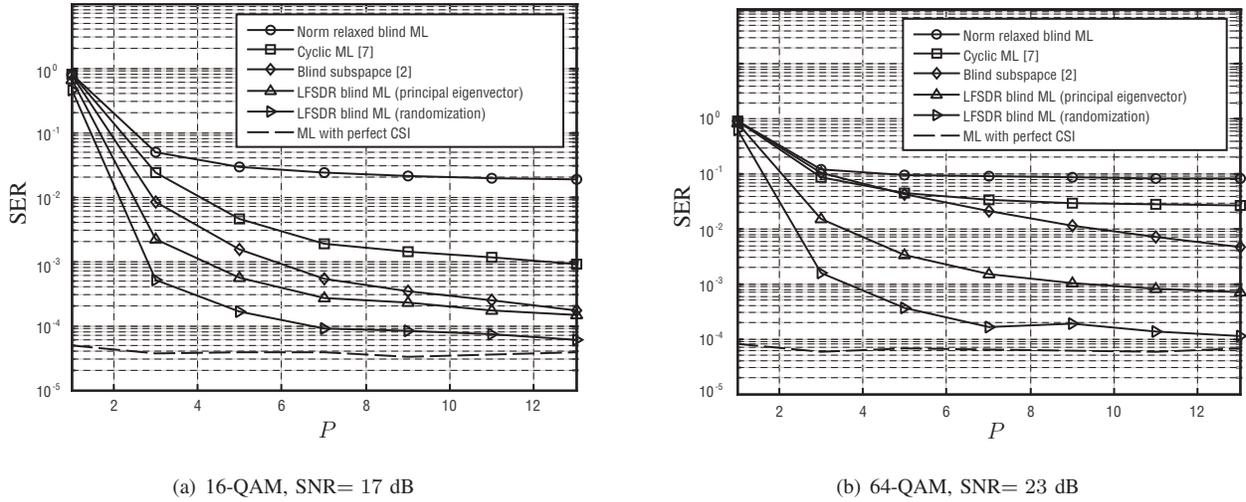
**Fig. 2.** Performance (SER v.s.  $P$ ) comparison results of the proposed LFSDR blind ML detector with some existing methods for the complex  $3 \times 4$  OSTBC.
