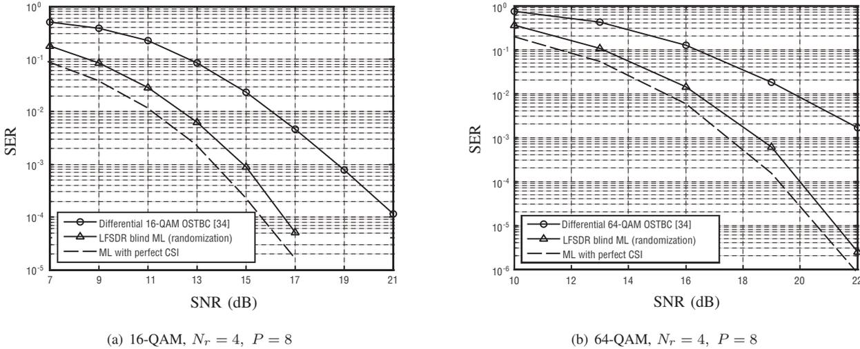
**Fig. 3.** Performance (SER v.s. SNR) comparison results of the LFSDR and the differential OSTBC scheme for the complex  $4 \times 4$  OSTBC.
