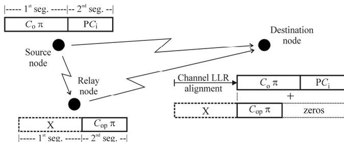
Fig. 1. Coded cooperation scenario with one cooperating relay.
