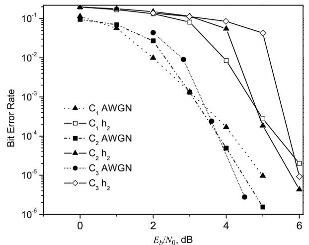
Fig. 4. Performance results for the turbo equalizer using a turbo SPC-TPC decoder.  $C_1 = (6, 5)^3$ ,  $C_2 = (10, 9)^3$ ,  $C_3 = (17, 16)^3$ ,  $h_2 = [0.407 \ 0.815 \ 0.407]$ .
