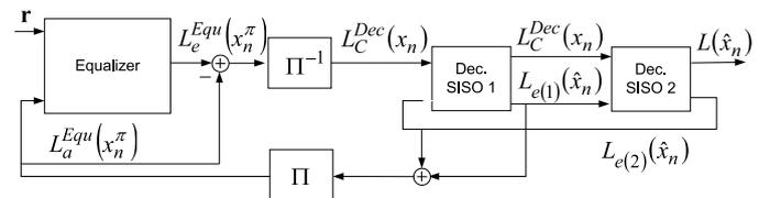
Fig. 2. Turbo Equalization using a 2D SPC-TPC code.
