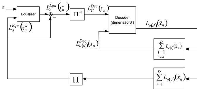
Fig. 3. The Novel Block Turbo Equalizer structure.
