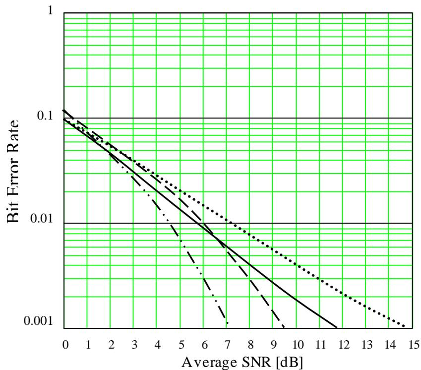
**Fig. 4** – Performance of the Multicarrier DS-CDMA system in a multipath Rayleigh fading channel
