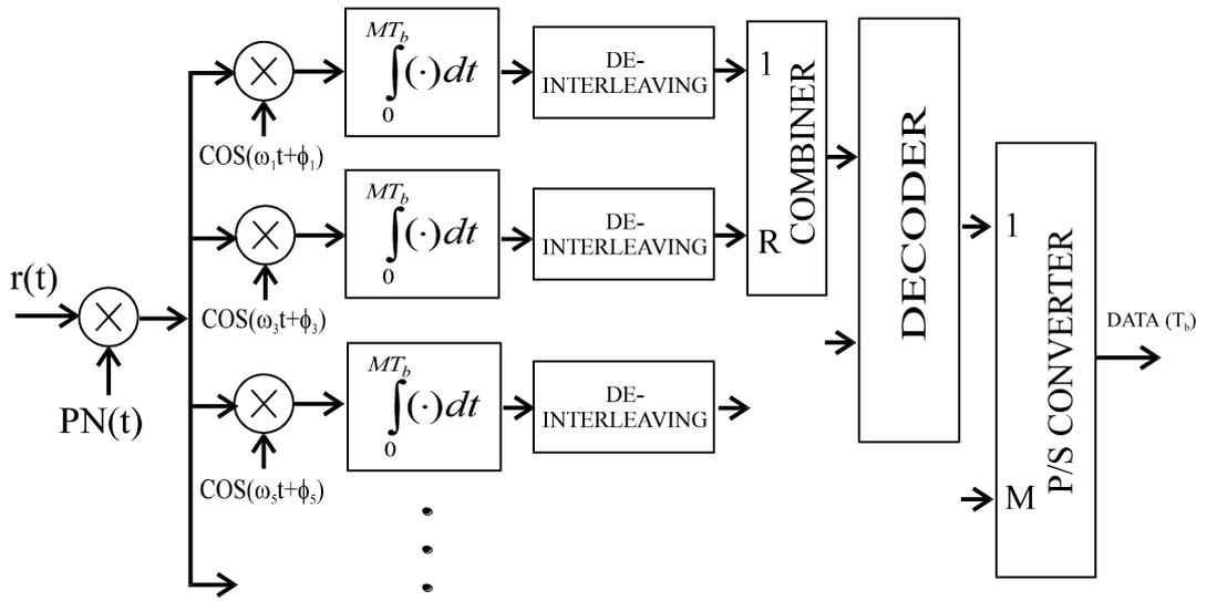
**Fig. 2** – Block diagram of the receiver of the coded Multicarrier DS-CDMA system
