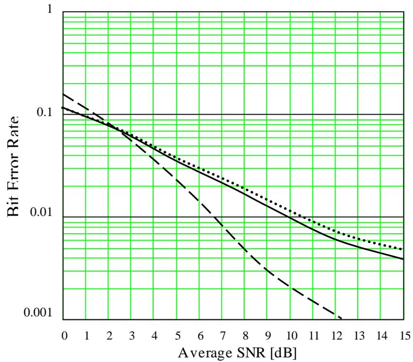
**Fig. 3** – Performance of the Multicarrier DS-CDMA system in a multipath Rayleigh fading channel
