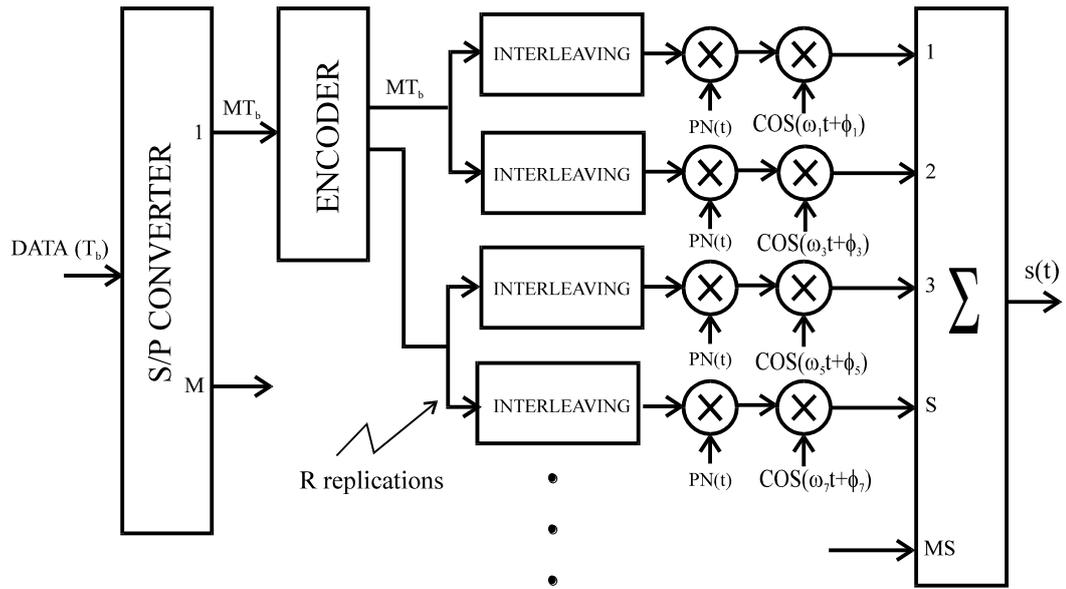
**Fig. 1** – Block diagram of the transmitter of the coded Multicarrier DS-SS-CDMA system
