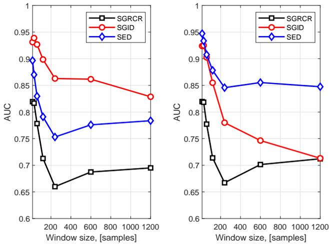
Fig. 1. AUC versus window size ( $S_w$ ): uniform signal and noise powers (left), nonuniform-dynamical signal and noise powers (right). The smallest window size is  $S_w = W_p = 15$  samples; the largest is  $S_w = n = 1200$ .
