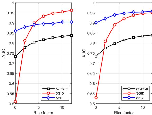
Fig. 2. AUC versus Rice factor ( $K$ ): uniform signal and noise powers (left), nonuniform-dynamical signal and noise powers (right).
