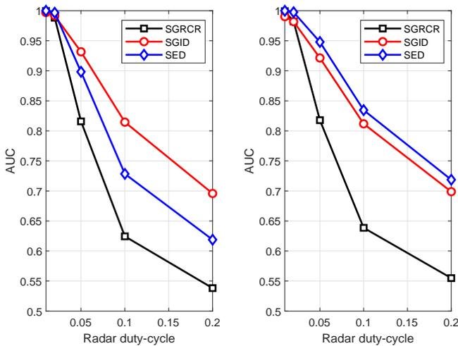
Fig. 5. AUC versus radar signal duty-cycle ( $D$ ): uniform signal and noise powers (left), nonuniform-dynamical signal and noise powers (right).
