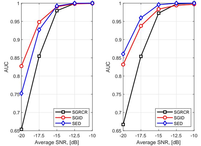
Fig. 3. AUC versus average SNR over all SUs: uniform signal and noise powers (left), nonuniform-dynamical signal and noise powers (right).
